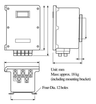
Figure 5. Converter Dimensions
